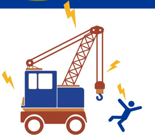
If a crane on the back of a truck touches a live powerline, the whole crane becomes electrified and anybody then touching that crane could be seriously injured or killed.
